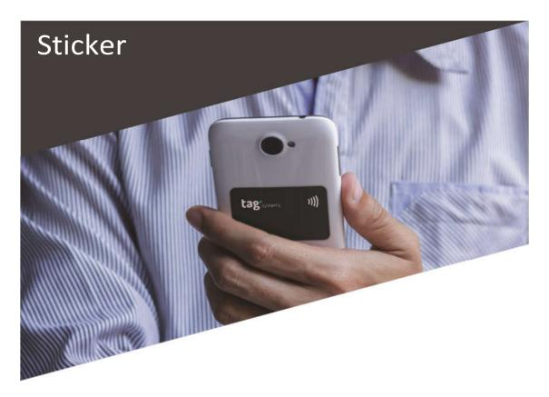
Tag Systems' Contactless Payment Stickers turn any mobile handset into a contactless EMV payment device, without any need for a handset or system upgrade.
